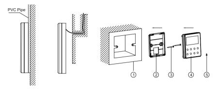
Fig.1.1 Accessories for the Installation of the Wired Controller
