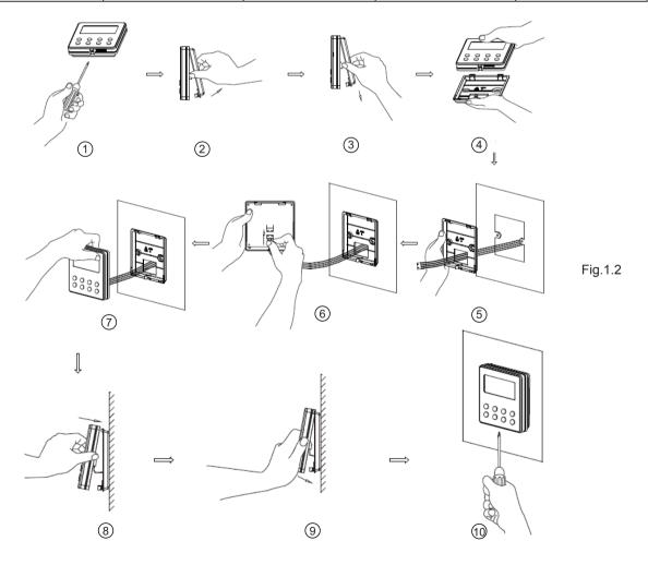
Fig. 1.2 shows the installation steps of the wired controller, but there are some issues that need your attention.
