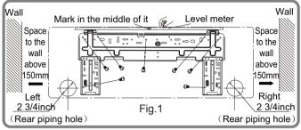
(2) Open a piping hole with the diameter of 2 3/4inch on the selected outlet pipe position. In order to drain smoothly, slant the piping hole on the wall slightly downward to the outdoor side with the gradient of 5-10°. (As show in Fig.2)
