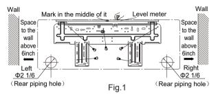
(2) Open a piping hole with the diameter of 2 1/6inch on the selected outlet pipe position. In order to drain smoothly, slant the piping hole on the wall slightly downward to the outdoor side with the gradient of 5-10°. (As show in Fig.2)
