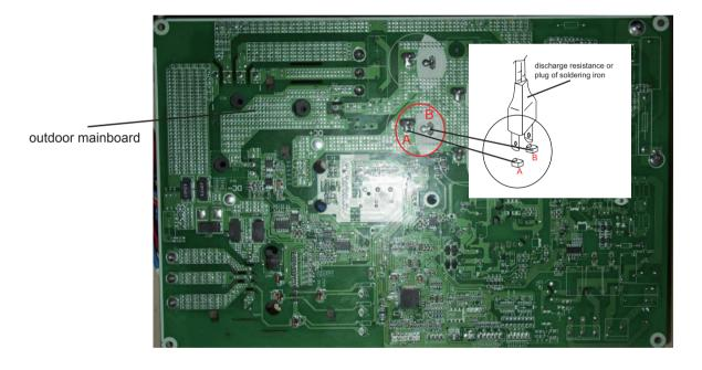
(3) After finish discharging electricity, measure the voltage between point A and B with universal meter to make sure if electricity discharging is completed, in order to prevent electric shock. If the voltage between the two points is below 20V, you can perform maintenance safely.
