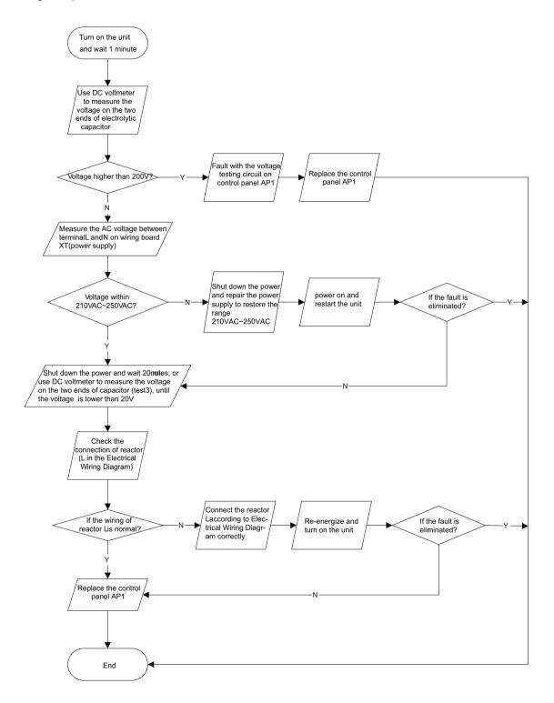
3.IPM protection, desynchronizing malfunction, phase current of compressor is overcurrent (AP1 below is control board of outdoor unit)
